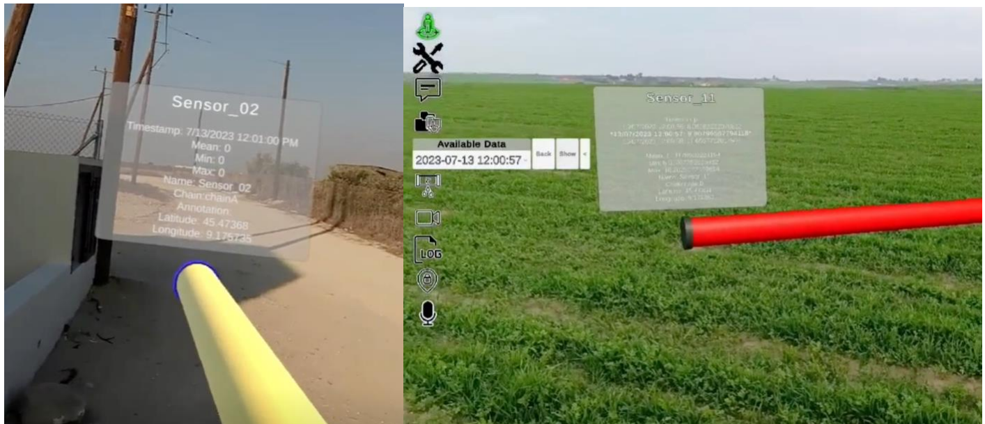
Figure 2 The image from the AR app displaying a 3D pipe overlaid with sensor information.
